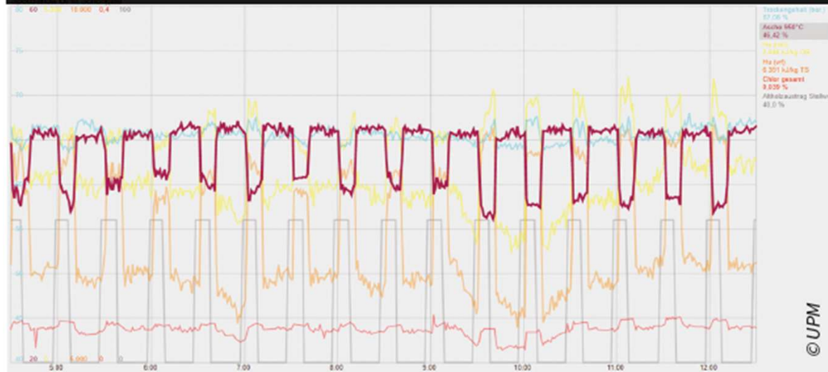
Figure 8: online heating value measurement during increased waste wood supply
